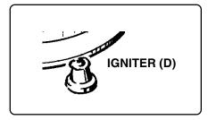
Each burner has an igniter (D) located on the burner plate. Keep the igniters clean. Avoid getting excess water or liquid cleaner on the igniter. If the igniter becomes too wet, it may continue to click but not ignite the burner. If the burner does not ignite in 4 seconds, turn off the control and wait until the igniter is dry.
